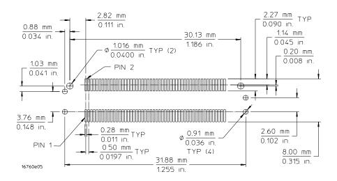
Board pad details for 100-pin Samtec connector and support shroud
